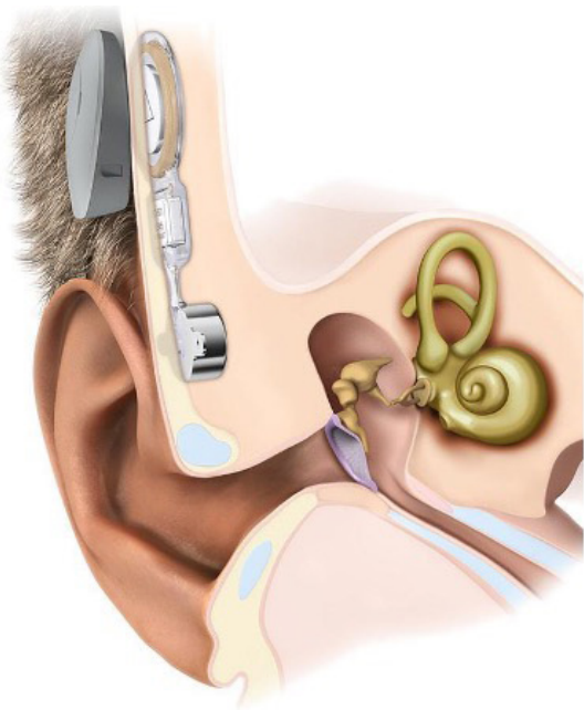
Figure 11.2: Illustration of an active BCHD. Source: Hearing Loss Association of America (2026)
