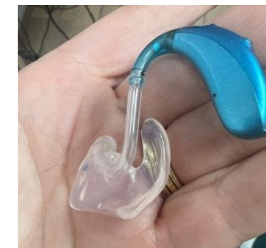
Figure 10.3: BTE HA with silicon ear mould.
