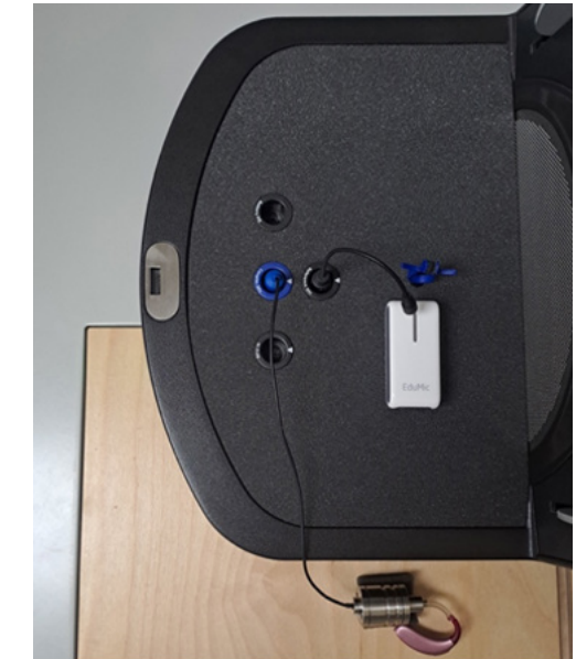
Figure 10.8: (a) RM transmitter outside the HIT, switched on, (b) RM transmitter inside the HIT, switched on
