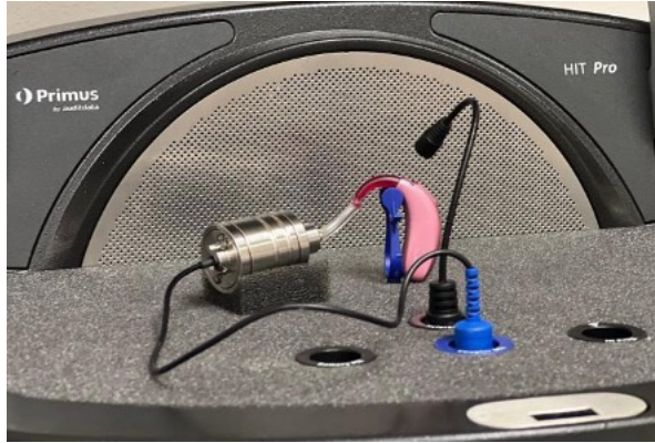
Figure 10.7: Hearing aid set-up in the test box
