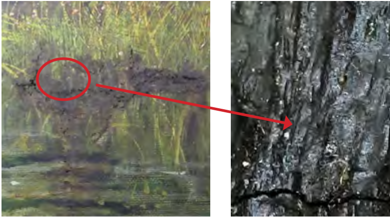
Figure 44: Bitumen-like substance from restorative patchwork. To the right is what it looks like under 10x microscopic magnification (photograph by Hannes Elsenbroek)
